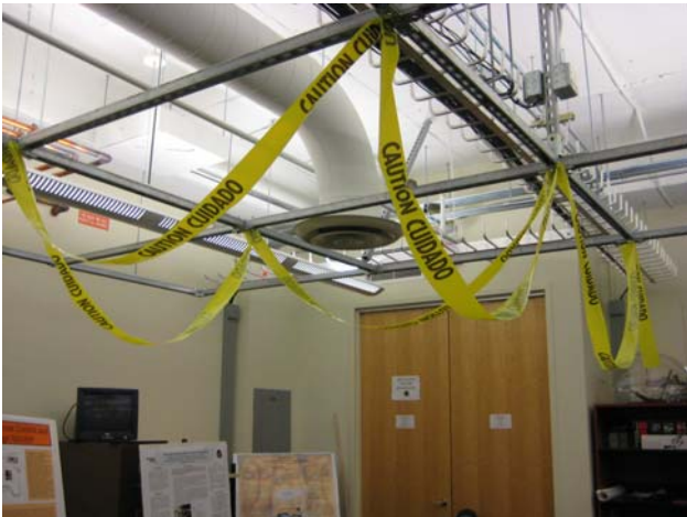
Figure 9: A preliminary method of marking the track for the blind condition by looping tape. Discarded due to lack of directional context at track intersections.
